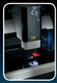
Component reports are produced with the aid of an OGP SmartScope CNC500 Vision System with six station touch probe and laser sensor, located within the climate controlled inspection area. For tool trials Precision Moulds has two Sumitomo Demag moulding machines in a dedicated mould shop adjacent to the tool manufacturing facilities.
